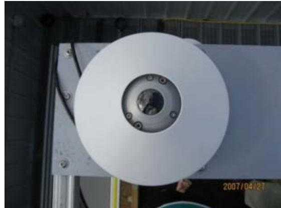
Figure 2 Kipp and Zonen CG4 pyrgeometer installed on roof tower.
